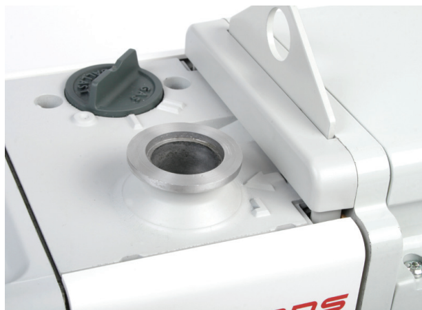
Figure 6.10: Gas Ballast control on Edwards RV oil-sealed rotary vane pump
