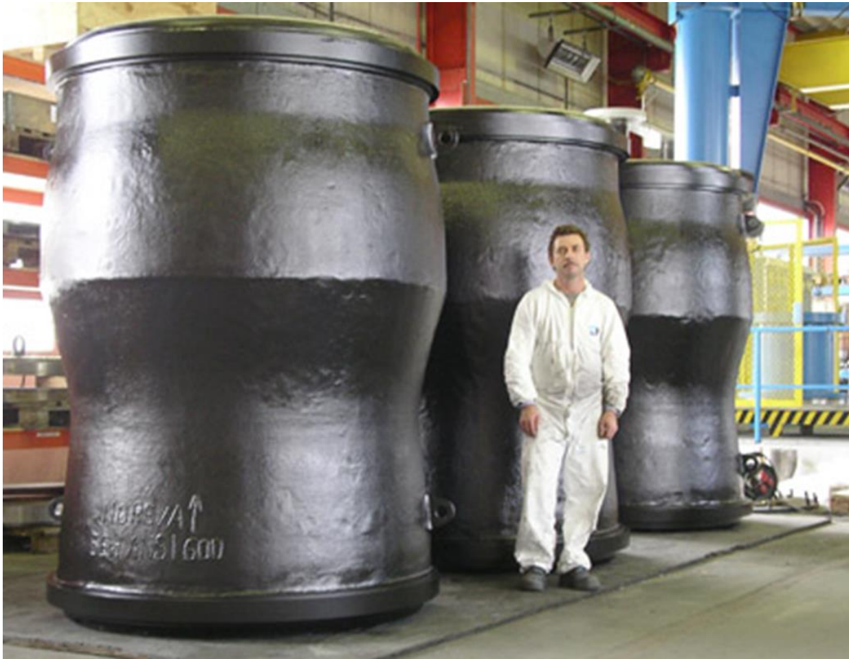
NB 56in class 600 welding ends, Water Transmission Project in Saudi Arabia
