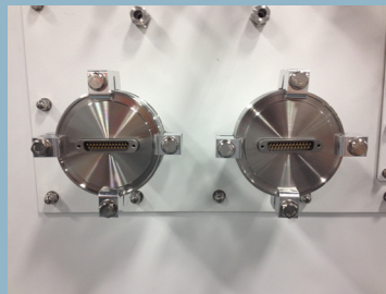
Sub-D 25 mounted on ISO-CF Flanges
