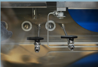
Media feedthroughs with specific length
