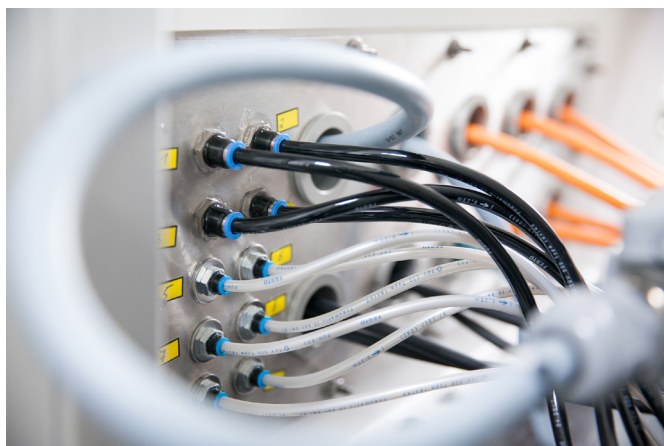
Special feedthroughs for equipment integration
