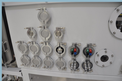
Glovebox rear wall with flanges and windows
