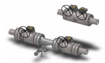
The antiquated system to achieve double block & bleed features is the use of 2 block valves and a spool piece with bleed valve. This configuration requires a lot of space and the operation of 2 valves, which especially in the actuated version is a very expensive and maintenance-intensive solution.
