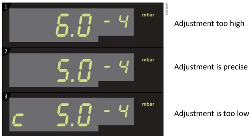
Figure 13 Zero adjustment for the PRG gauge head
