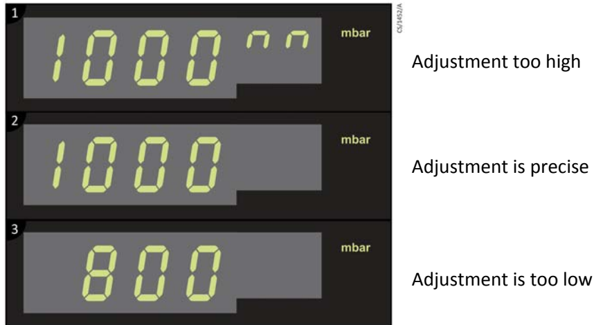
Figure 12 Full-scale adjustment for the PRG gauge head
