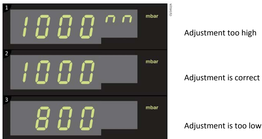
Figure 11 Full-scale adjustment for the PRG gauge head
