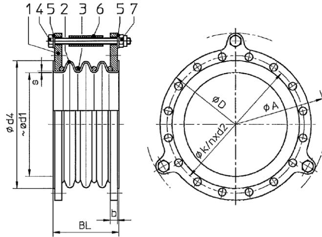
Fig. 1 FLUROFLEX®-N 1 to 6
