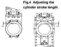
Pneumatic cylinder type EC and ECS for knife gate valves
