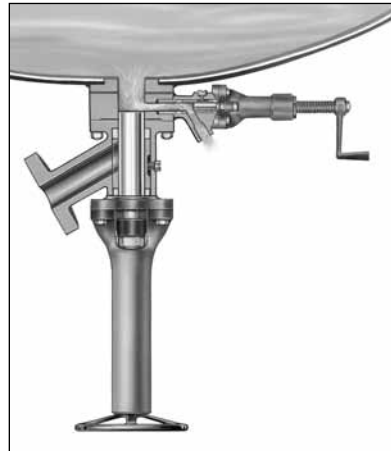
Fig. 2 - Drain Valve Open for Sample
