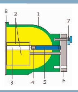
The shielding container consists of a cast-steel leadfilled Housing. A rotary Lockable Shutter is provided to close the radiation outlet channel. The shutter is rotated by a Handle which is secured in the open or closed position by a padlock.\* The Source Holder is protected against unauthorised access by the Handle.
