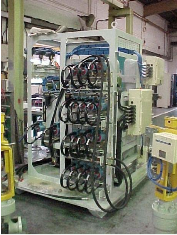
Pictures show Explosion Proof (Eex-d) HPU and control system provided by Copes Vulcan on a recent contract.
