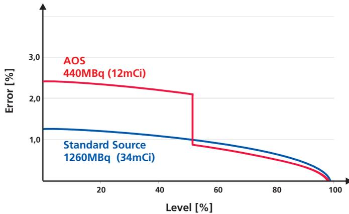
In this example the accuracy at the operating point is given with 1%. Considering the mould size and wall thicknesses, following source activities were determined for a Co-60 rod source:
