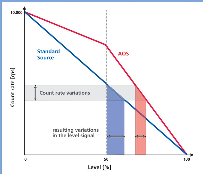
The bottom measuring range is characterized by a significantly reduced source activity. The AOS provides sufficient counts for a reliable measurement during the start of casting.
