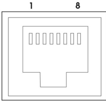
Socket connection FCC68/RJ45 Type 8 way
