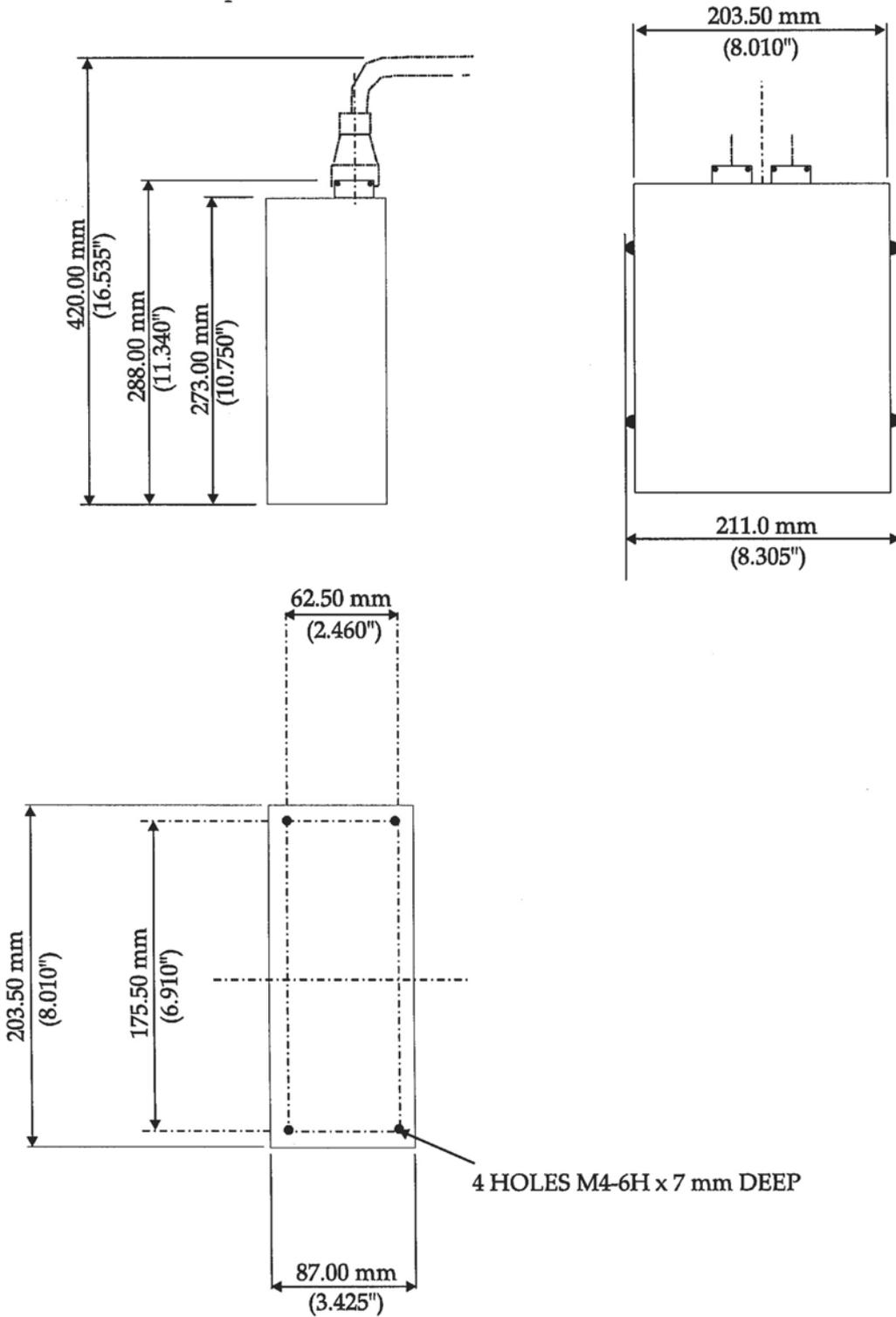
Figure A9 - Rack mounting dimensions
